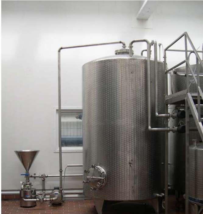
The new juice concentrate tank at Harboes Brewery - the powder mixer to the left. The ISO-MIX rotary jet head is placed inside the tank and can not be seen at the photo
